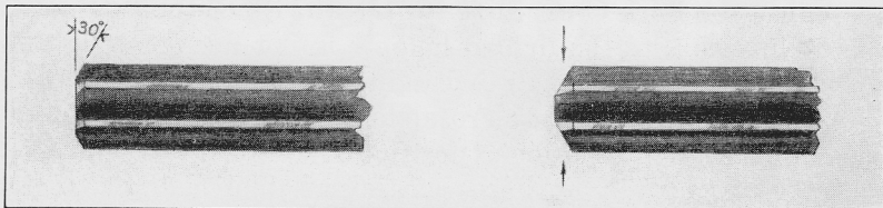
Fig. 14. Grind away the reamer nose when resharpener
